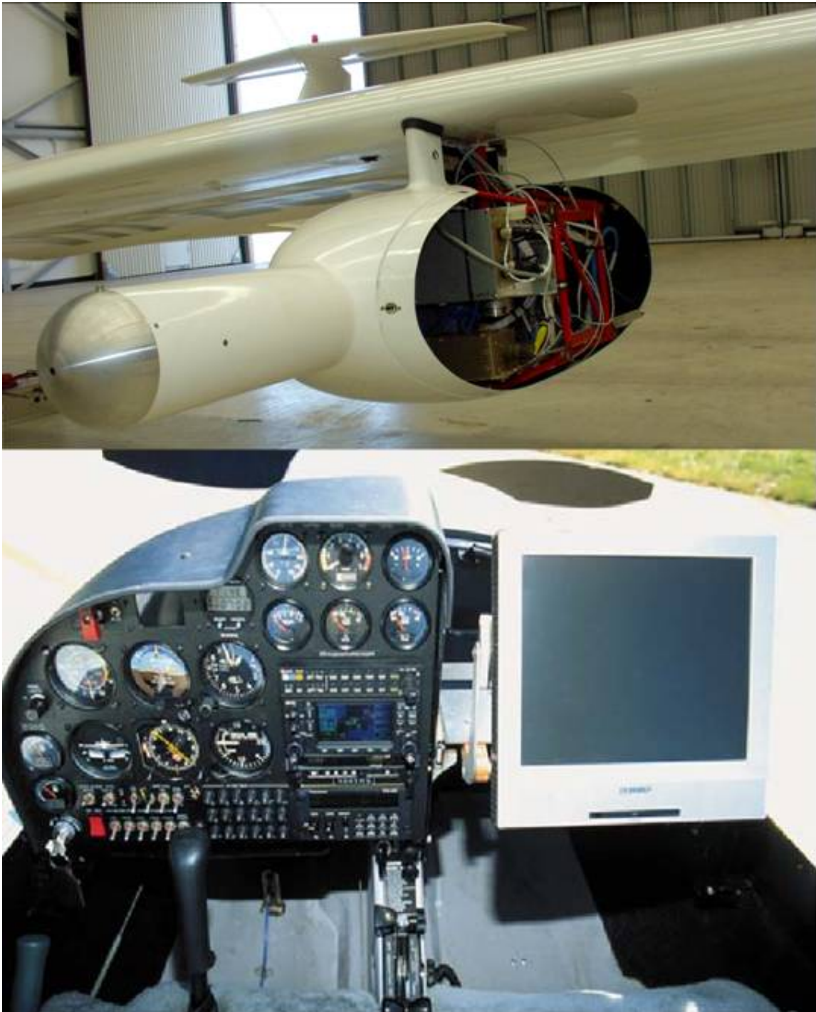
Figure 6. View of one of the underwing pod with the cover off, and view of the cockpit showing cockpit computer display.
