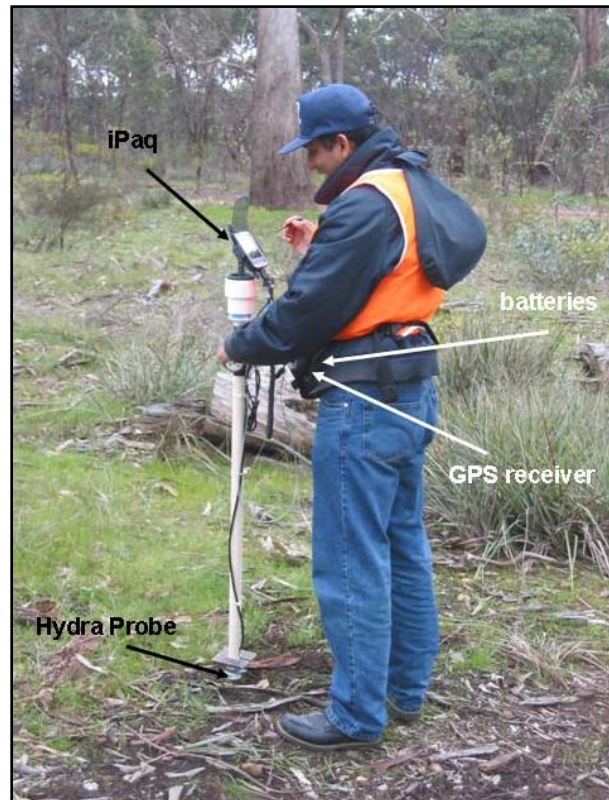
Figure 42. Typical set up of a soil moisture measuring unit, with hydra probe communicating directly to an iPAQ and a wireless GPS receiver. Everything is powered by a battery carried by the user.
