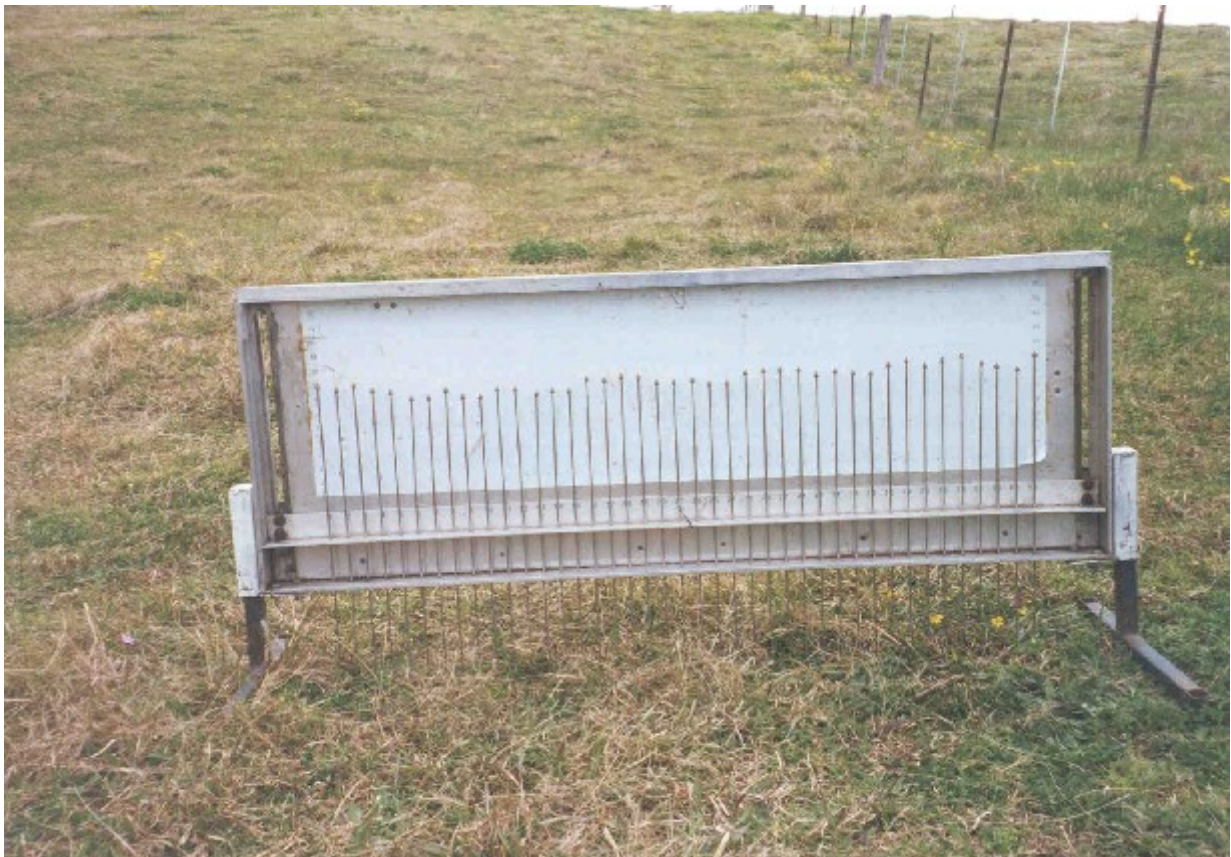
Figure 43. Pin profiler for surface roughness measurements
