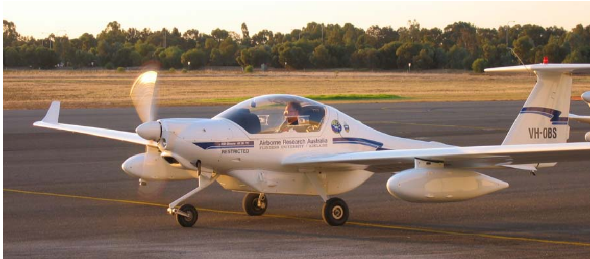
Figure 4. The Diamond ECO-Dimona aircraft with PLMR mounted under the fuselage, and thermal imager, digital camera and NDVI scanner in an underwing pod.
